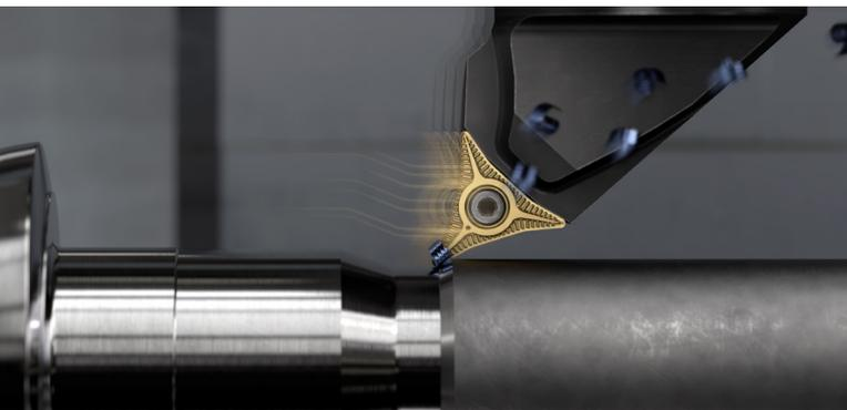
CoroTurn Prime – as cutting is performed in the direction moving away from the shoulder, there is no danger of chip jamming.
