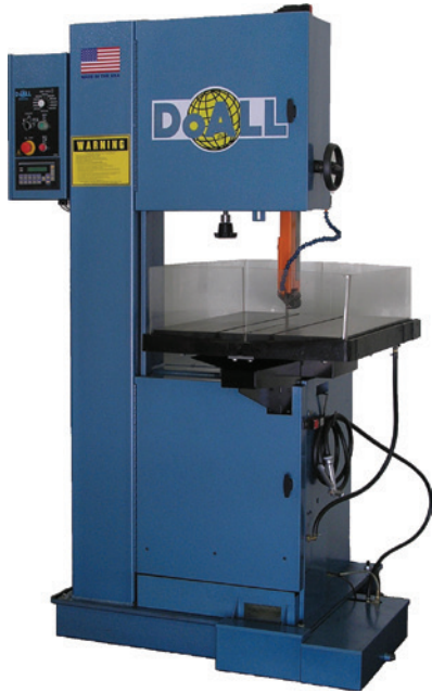
DoALL 2012-D12 Diamond Saw – 20 x 12" Capacity
