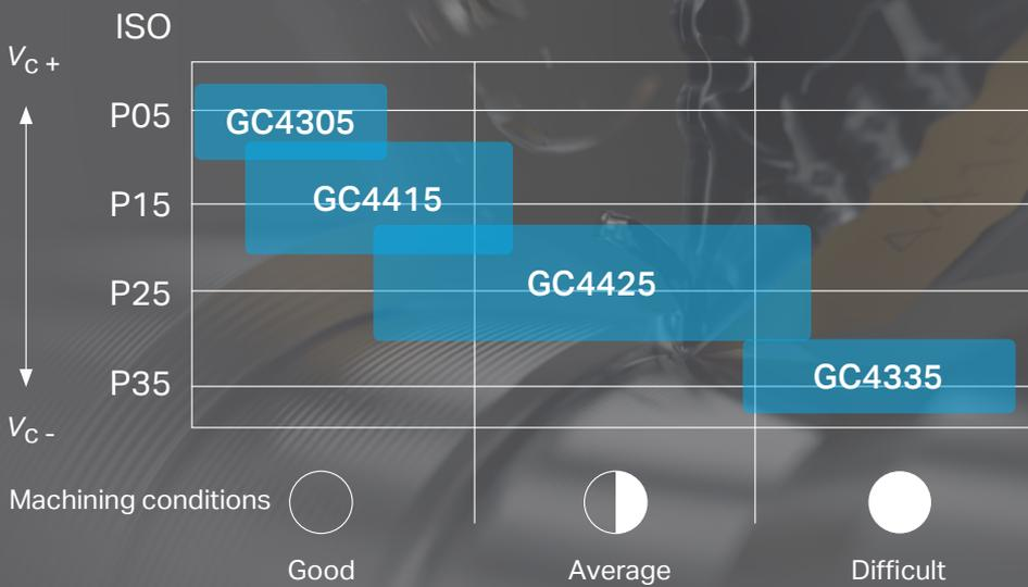
First choice grade GC4425 delivers improved wear resistance, heat resistance and toughness, significantly expanding the application range.
